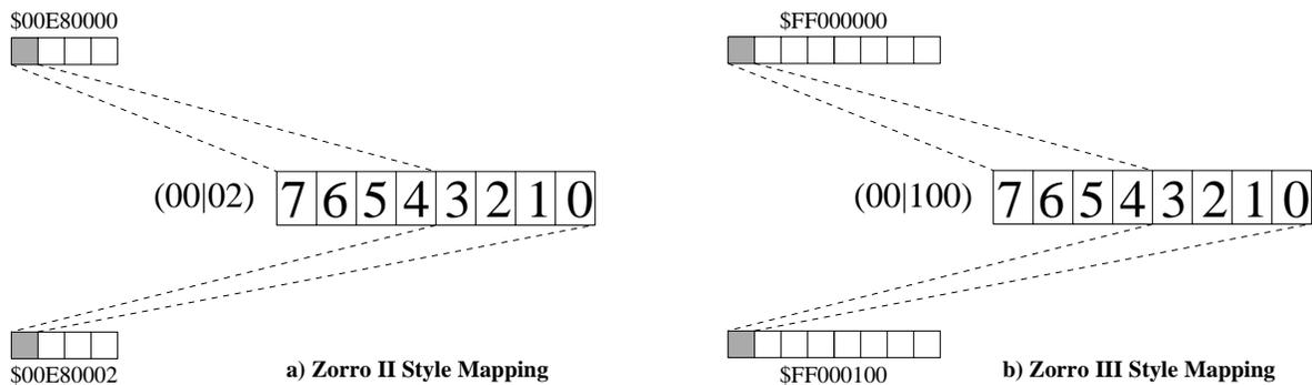
Figure 8-1: Configuration Register Mapping
